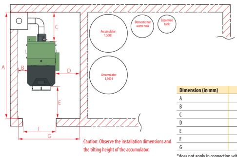
Minimum ceiling height: 2.00 m Recommended ceiling height:: 2.30 m
