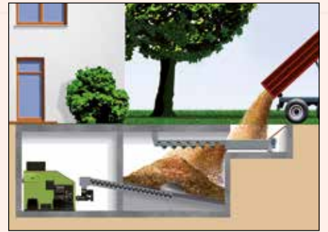
Example: fuel storage room in cellar with screw transfer system for filling via light shaft
