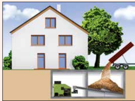
Example: fuel storage room created underground with load-bearing ceiling
