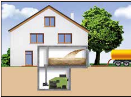
Example: pellet storage room with injection mechanism
