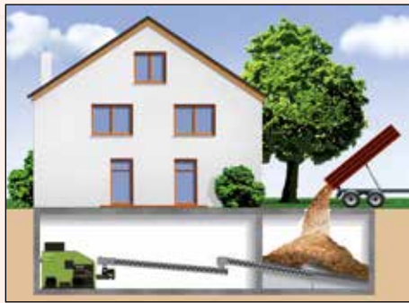
Example: fuel transported via second conveyor auger from fuel storage room located some distance away
