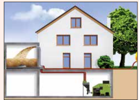
Example: fuel storage room away from boiler room – pellets transported using HDG pellet suction system
